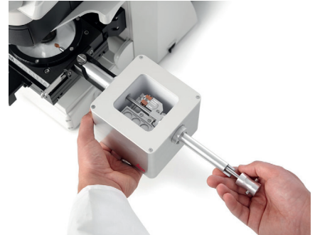
Loading of a grid cartridge into the THUNDER Imager EM Cryo CLEM using the transfer shuttle
