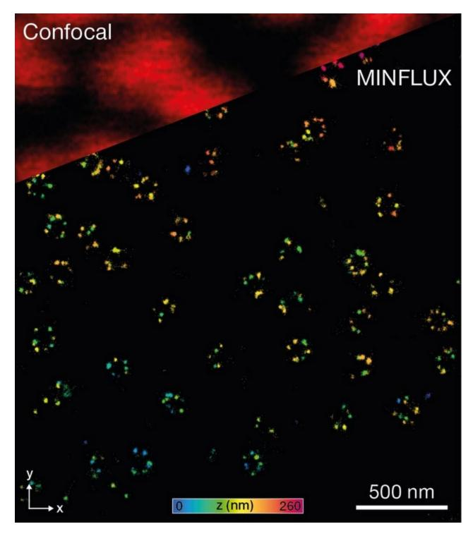
Figure 1. Confocal and 3D MINFLUX images of a nuclear pore complex sample.
