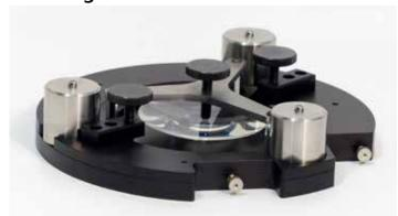
This micrometer transfer stage allows the examination of a sample with an inverted optical microscope, where the sample faces down, and with AFM, where the sample faces up. The sample – a glass lens – is fixed in place after the area of interest is located using the optical microscope and then flipped over and transferred to the AFM with a repositioning accuracy of better than  $10\mu m.$
