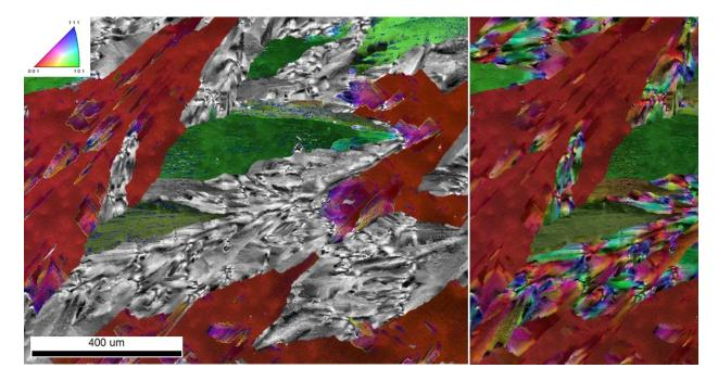
Figure 1: Recrystallised fraction separation in the gold layer in an electronic component.
