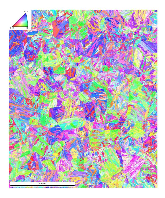
Figure 2: Reconstruction of original high-temperature austenite microstructure from martensitic measurement.
